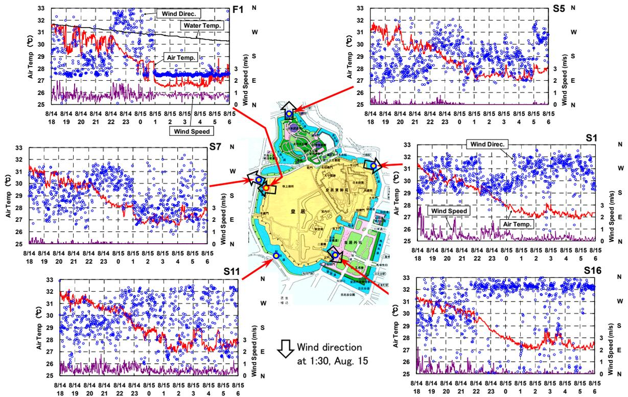
Fig.2 Seeping-out phenomena of cool air in calm night—1-minute average time variations of air temperature, wind speed and direction at boundary points.
